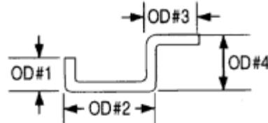
To establish the flat blank size required, add all outside dimensions (OD), then subtract twice the bend allowance (BA) times the number of 90 deg. Bends.
