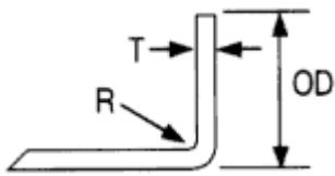
To establish gauge setting dimension, subtract bend allowance (BA) from desired outside dimension on finished part (OD)
